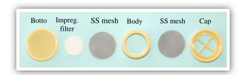
1. Wash all parts of passive samplers by tap waters. Rinse twice by deionized water. Dry on the air. Do not dry by heat.
