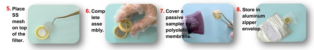
Wear glove when working with passive samplers. Assembly should be done in clean air to avoid contamination.
